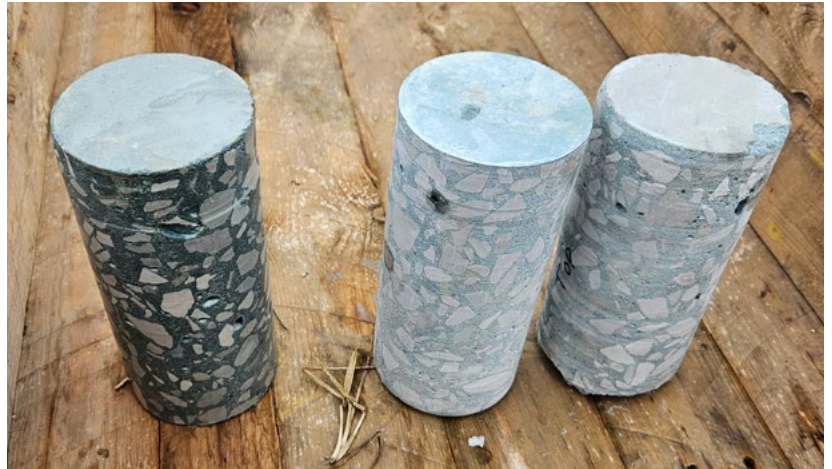
Cores were taken from each panel to verify in-situ compressive strength.
